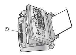
**9** Reinstall the drum and toner unit (1) by holding the tabs.
